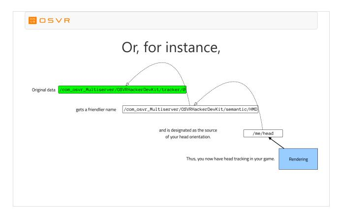
As a final example and a bit of a tease, here's the diagram showing how the rendering engine in your game gets head tracker data from the OSVR HDK's integrated orientation tracker.
