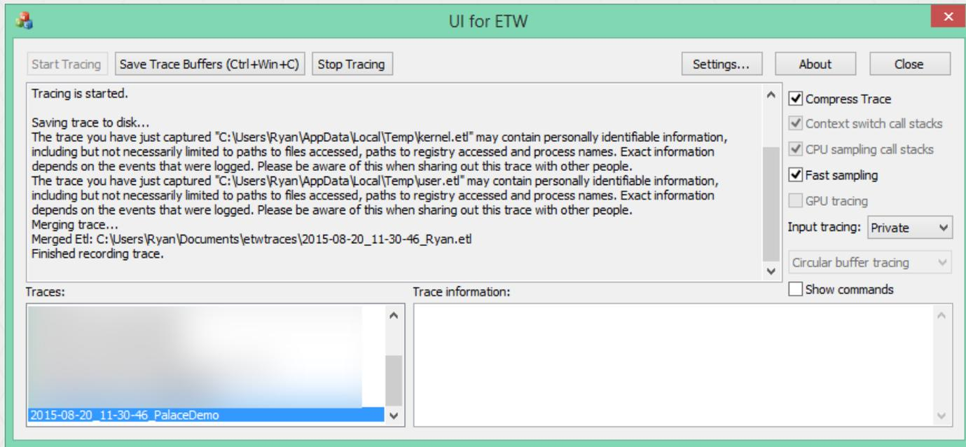
Settings I used for this trace: I chose to turn on fast sampling, but not GPU tracing, and traced to an in-memory circular buffer that gets saved on a keystroke. This can let you leave tracing running continuously, then after you notice unusual behavior or something you'd like to investigate, you can hit the shortcut key and save a trace of the last  $x$  seconds, for after-the-fact performance investigation.
